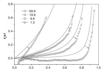
**Figure 3.** Pairs of force-extension curves of semiflexible chains of N = 100 and the stiffness ratio  $L_c/I_p$  given in the legend computed from simulations at isometric conditions (symbols) and from the WLC interpolation formula (Equation 1).
