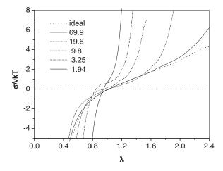
**Figure 5.** Stress-strain relations of the three-chain model networks computed for stiffness  $L_c/I_p$  given in the legend (in the order from right to left). The ideal network relation is shown by the dotted line.
